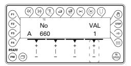
VAL ● By pressing the corresponding +/- key set the desired value for the parameter selected, e.g. "2" for the "bobbin rest thread counter on" function.
