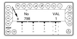
VAL ● By pressing the corresponding +/- key select the desired user level:
