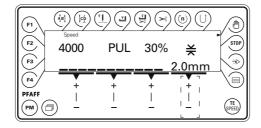
₹ • Enter the feed stroke by pressing the corresponding +/- key.
