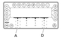
Press and hold "+" on keys A and D and switch on the machine.
