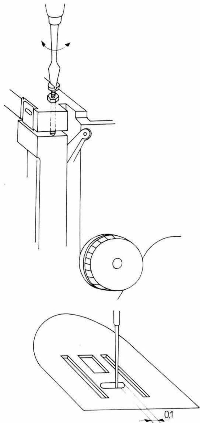
Table 6 Adjusting the frame stop screw
