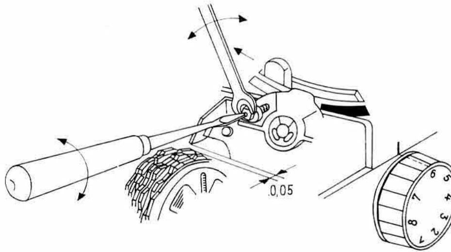
Table 4 Adjusting the rear feeling lever to pattern position 6 with Kl. 8014/39 and to pattern position 2 with Kl. 8014/40
